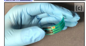
Prof. HJ Cho's fabricated pseudo-reference electrode on a flexible substrate for heavy metal ion detection
